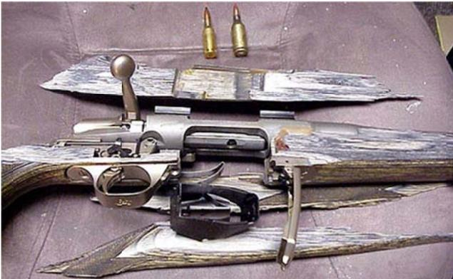
There were IMMENSE pressures in that one. It managed to get the .243" diameter bullet out of the barrel by squeezing it down to .224", but the resulting pressure caused the rifle to come apart. It even blew the stock into three pieces! The shooter wasn't seriously hurt, but he could have been!
